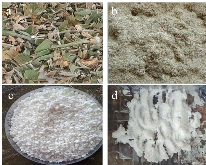
Figure 2. Physical appearance of (a) Chopped Typha angustifolia , (b) Crushed Typha angustifolia , (c) Isolated cellulose and (d) Cellulose nanocrystals.
