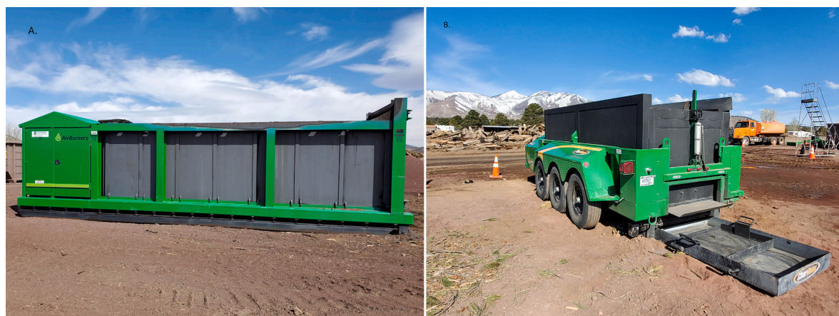
Fig. 4. (A) The roll-off FireBox S-119 Air Curtain Burner and (B) CharBoss used in the current study.
