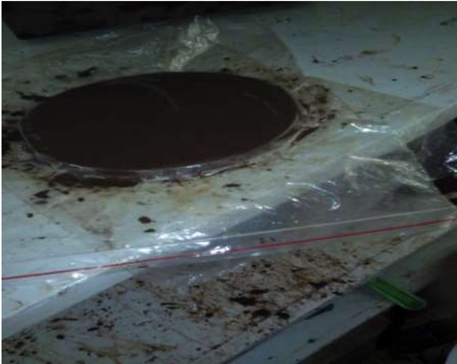
Figure8: filter removed from the female mold ready to be air dried
