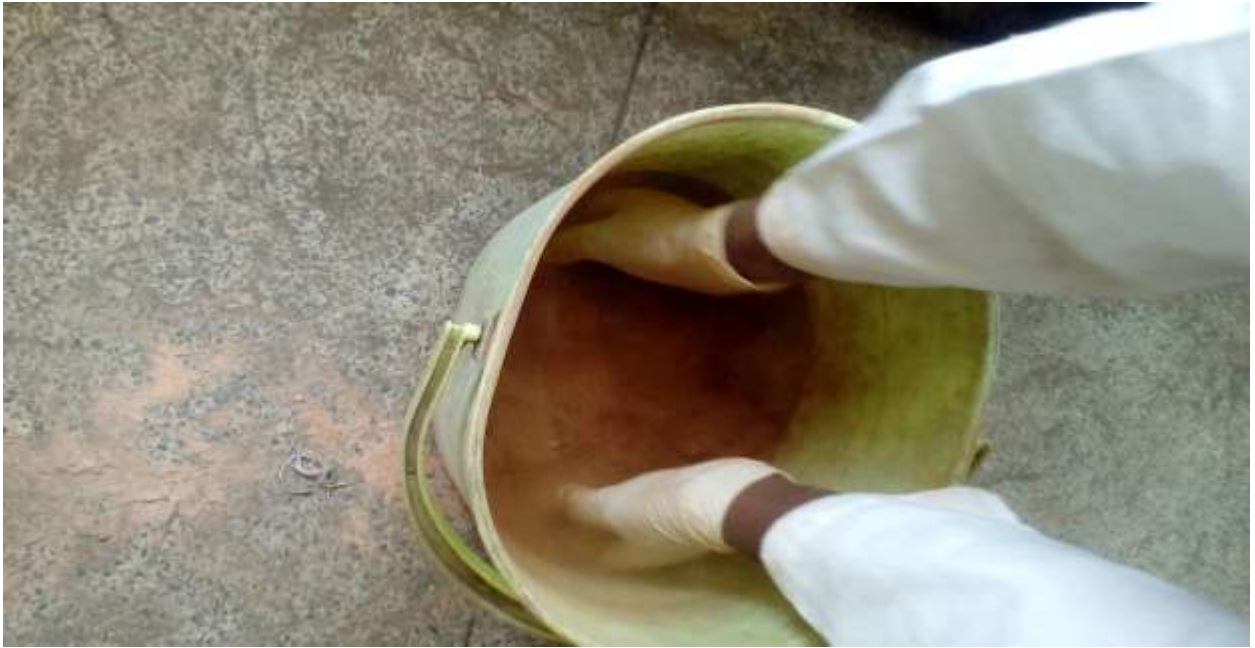
Figure 2 Preparing dry mix by rolling back and forth
