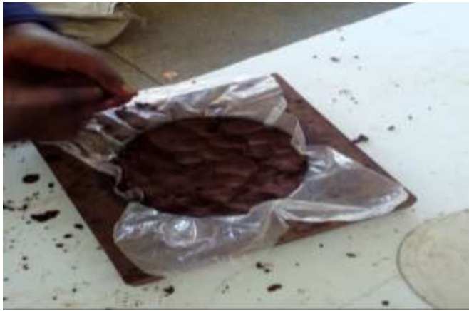
Figure 4: Dough placed in the female mold
