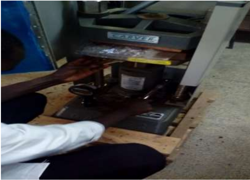
Figure 6: Pressing the wet mix to the disc shaped filters
