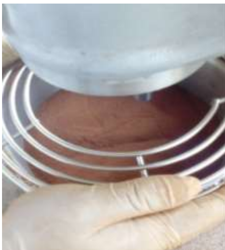
Figure 3: Thoroughly mixed Clay and sawdust mixture
