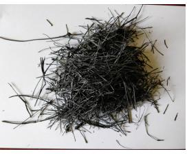
Grass Char prepared from trash and cut grass used to make bio char briquettes.
