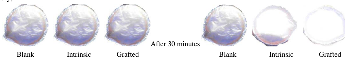
Fig. 8 Sewerage water samples ( C_1 ) which were barge in color but the samples in intrinsic and grafted ZnO decolorized after sunlight exposure.
