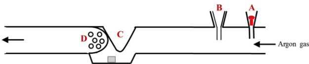
Fig. 2. A longitudinal cross-section of the modified glass tube used for annealing.
