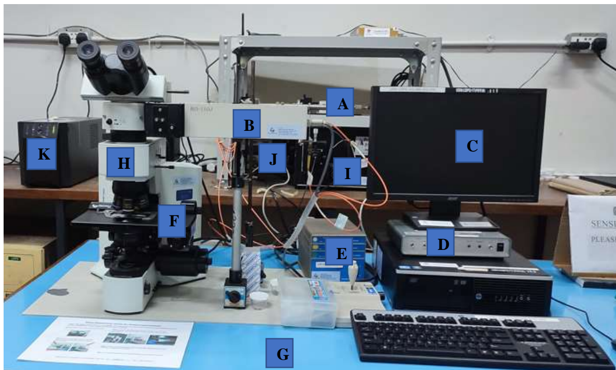
Figure 4.3: A photograph Showing the STR Raman Spectrometer system (Photo credits of the UON, Kenya). The part named A depicts 532nm laser, B- Raman optics system, C- 21.6-inch Acer LCD display, D- STR Raman controller system (CPU), E- The stage control system, F- Stage, G-Optical table H-Confocal Raman Microscope unit. I- Acton Sp2300 spectrometer system, J- Pixis 256 CCD Detector, K-UPS system.
