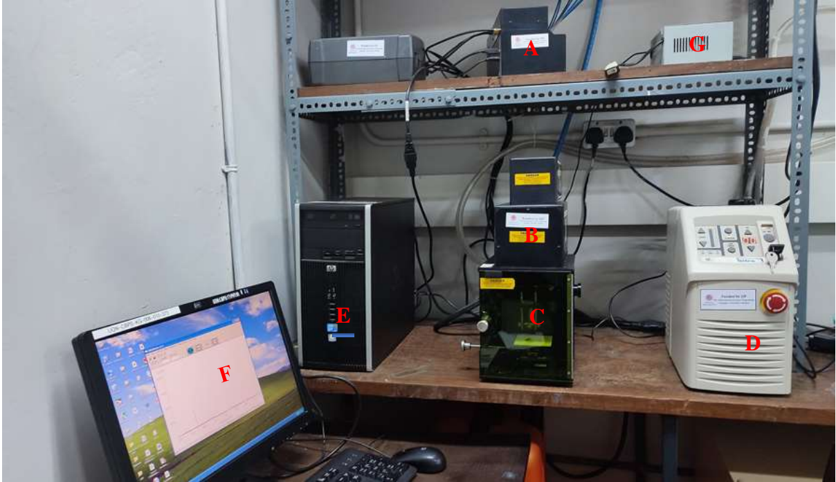
Figure 3.1: An image of LIBS2500Plus System (LIBS) which was utilized in this study (Photo credits to the Laser Lab, UON, Kenya). The Part named A indicates a spectrometer module, B- Big Sky Laser Quantel Laser, C- Sample analysis chamber, D- Laser power system, E- CPU, F-LCD monitor
